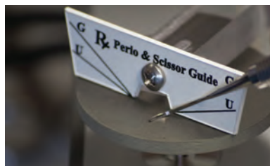
Figure 9: Utilize the proper guide to sharpen curettes on a mechanical device: “U” for Universal curettes and “G” for Gracey curettes.
