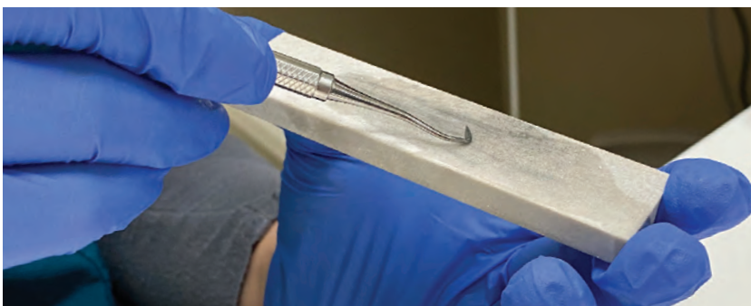
Figure 6: Bring the instrument 20 degrees off of parallel and move the stone back and forth with more force on the “down” stroke.
