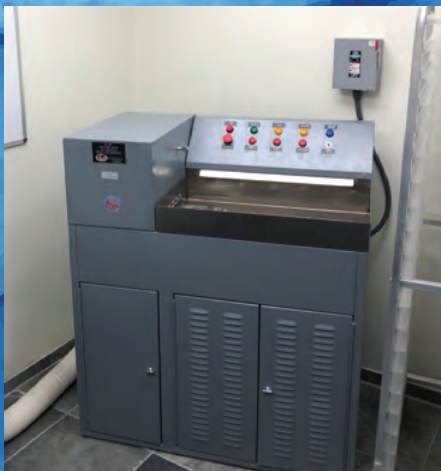
A pulverizer makes “ashes” from the dried bones.
